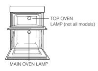
Warning: To avoid electric shocks - please ensure that the electricity supply to the appliance is switched off and the appliance is fully cold, before removing the lamp lens.
